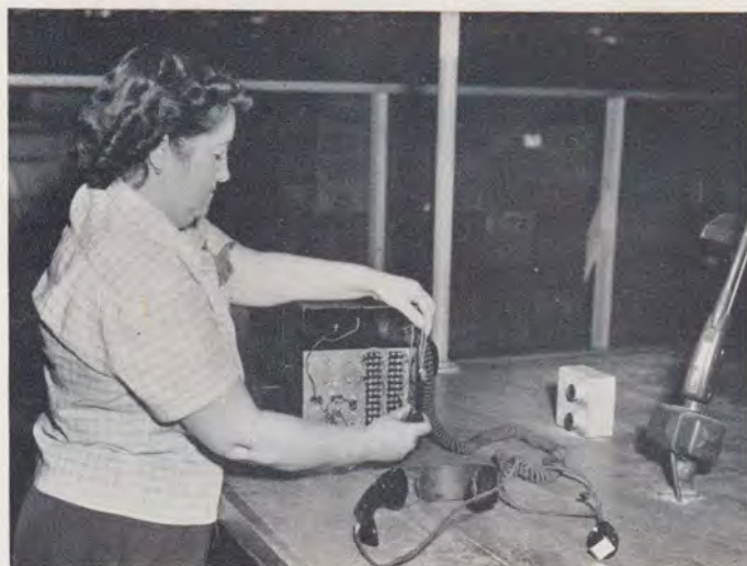
Agnes Baker of Western Electric's Indianapolis Works puts the final touches on one of the new Ground Observer Telephone sets that provide instant communication between Air Force Civil Defense Filter Centers and volunteer aircraft spotter posts.
