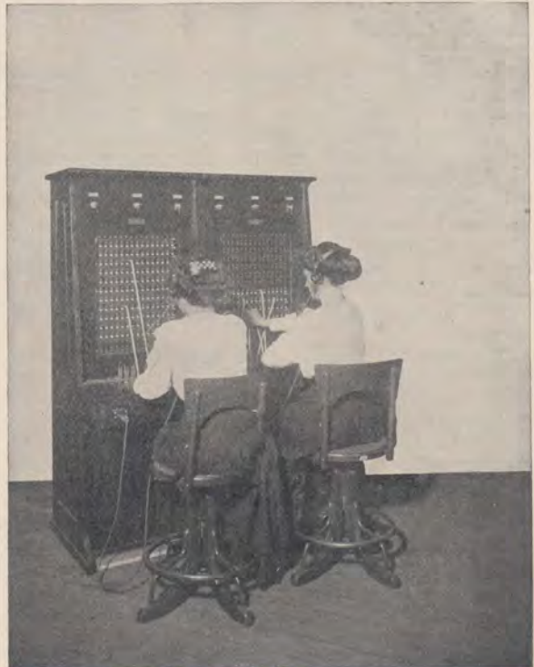
Private Branch Exchange for Business Houses and Hotels having much Telephone Service.
