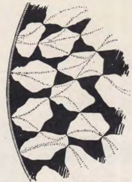
Fig. 3-B. But when the diaphragm springs back the grains are loosely packed and fewer electrons can pass from grain to grain through the chamber.
