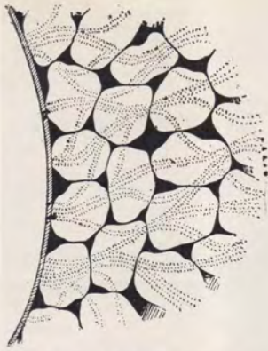
Fig. 3-A. Carbon grains in a transmitter magnified about fifty times each way. When the diaphragm is bent in, the grains are closely packed together and many electrons can pass through.
