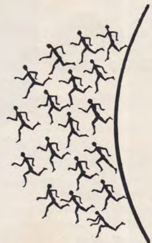
Fig. 6-B. When the diaphragm bows out, the molecules are pushed away. So these molecules rush back and forth just as do those shown in Figs. 2-A and 2-B.
