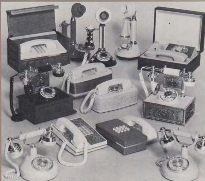
Design Line* telephones came in a wide variety of shapes and colors. While many of the housings were made by outside suppliers, Western continued through the 70s to supply all the inner workings.
