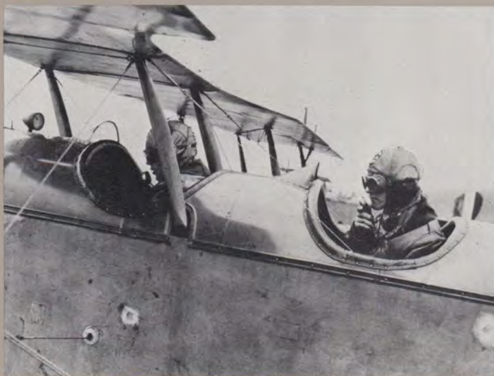
Early air-ground radio experiments conducted by Western Electric during World War I. Prior to the invention of the microphone, a passenger needed strong lungs to communicate with the pilot. Those are fabric patches, not bullet holes that are visible on the fuselage.
