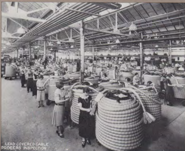
Women inspecting lead-covered cable at Hawthorne in 1930, looking for possible flaws in what was then the primary medium for telephone transmission.
