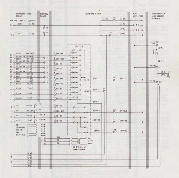
Fig. 15—Schematic, 836AM Telephone Set (Rotary Primary Station) (Sheet 2 of 2)
