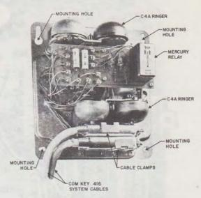
FIGURE 2. 24 A APPARATUS UNIT
