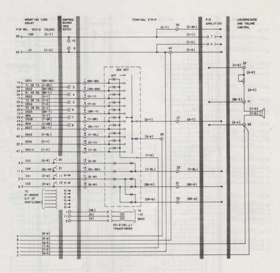
Fig. 17—Schematic, 2836AM Telephone Set (TOUCH-TONE Primary Station) (Sheet 2 of 2)
