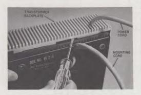
Fig. 5-Removing Transformer
