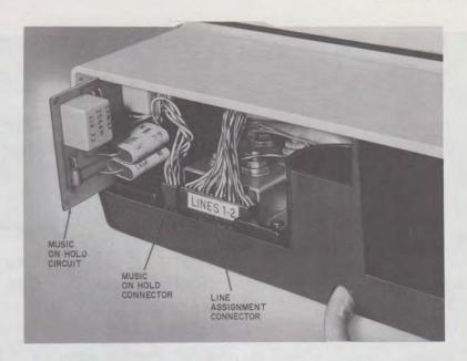
Fig. 6—Line Assignment Connector and Music-on-Hold Board
