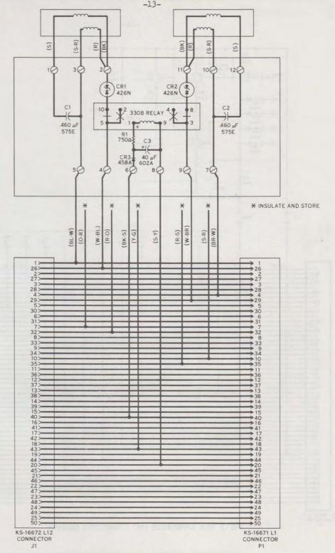
FIG. 12. 24A APPARATUS CONNECTING DIAGRAM
