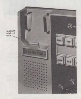
Fig. 9—Handset Hook Attachment for Wall Set
