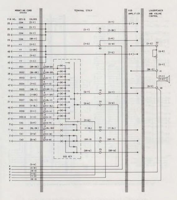
Fig. 16—Schematic, 837AM Telephone Set (Rotary Satellite Station) (Sheet 2 of 2)
