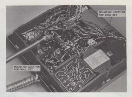
Fig. 8—Set Modification for Wall Mounting
