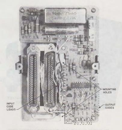
FIGURE 8. 26 A APPARATUS UNIT BASE
