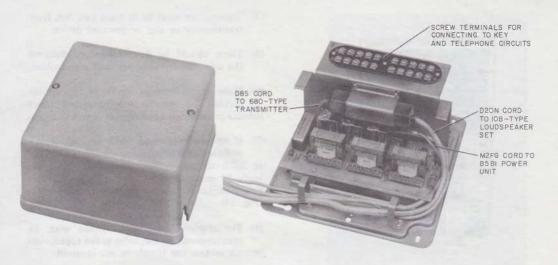
Fig. 7-80-Type Control Unit With Cover Removed
