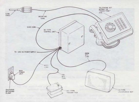
Fig. 2-Typical Arrangement of 4A Speakerphone System With 2- or 4-Wire Telephone Set
