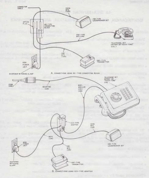
Fig. 1—Typical Arrangements of 4A Speakerphone System
