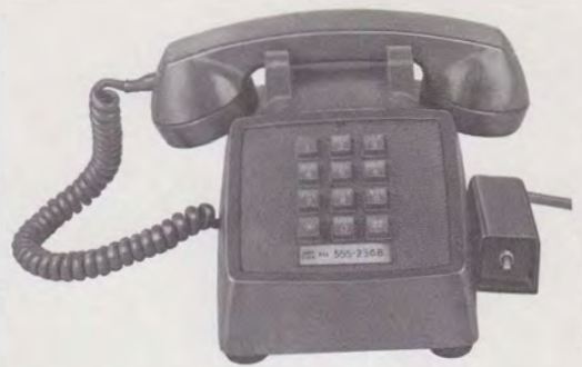
Fig. 7—KS-21254 Type Key Installed With 2500-Type Telephone Set Using 77A Mounting Bracket
