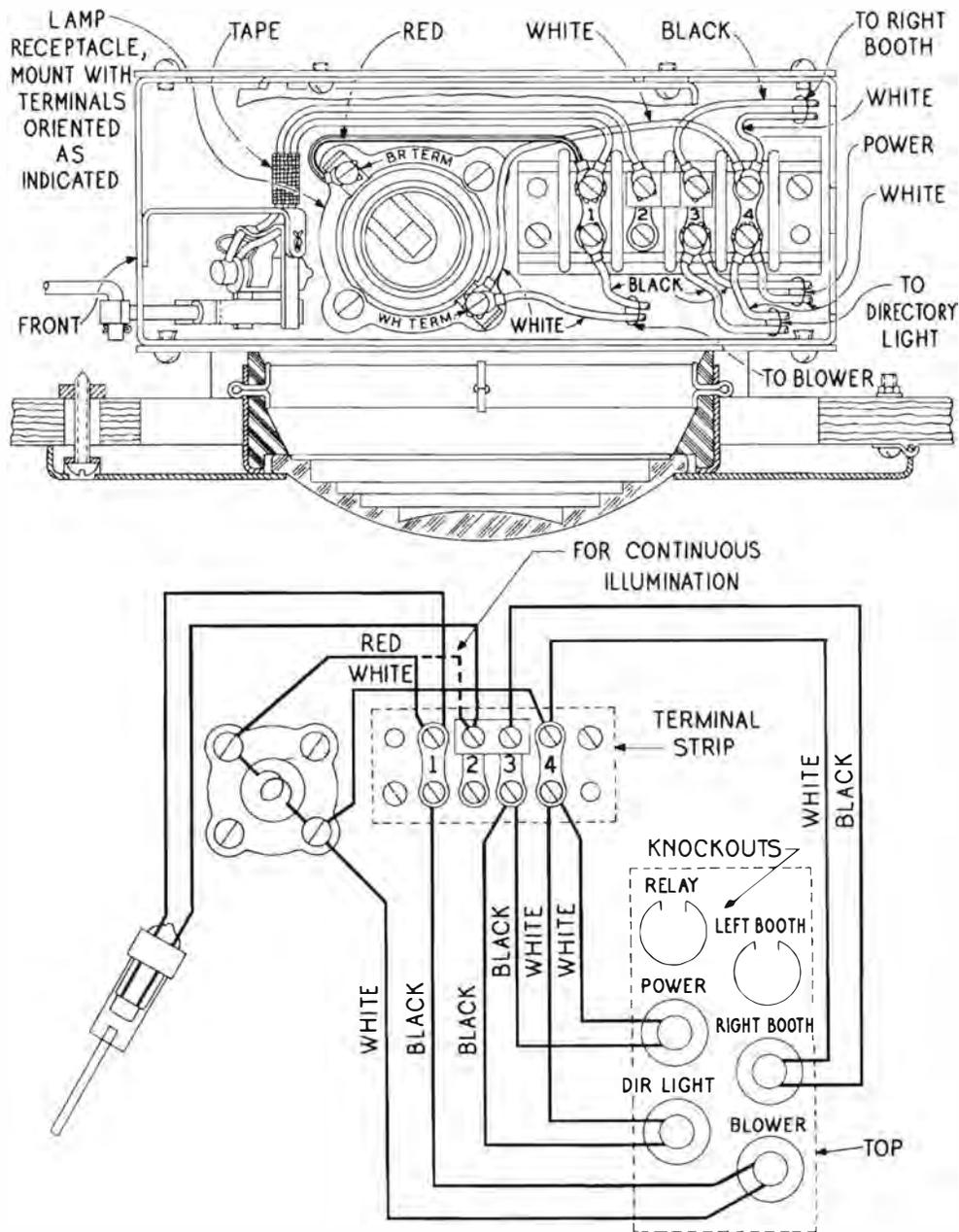
Fig. 9 - 4A Light Fixture for Four Cables
