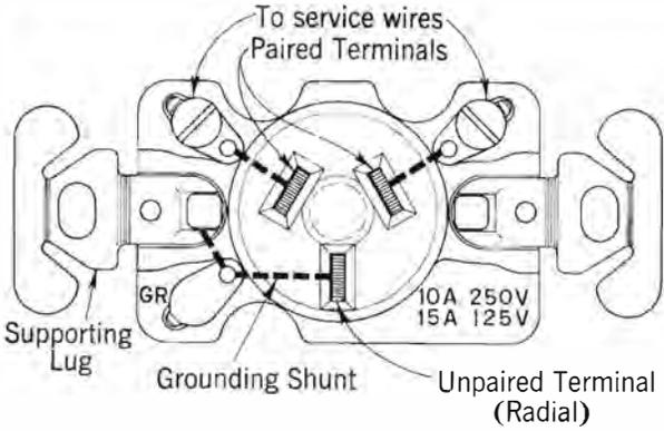
◀ Fig. 1 - 3-wire Flush-type Receptacle with Grounding Shunt
