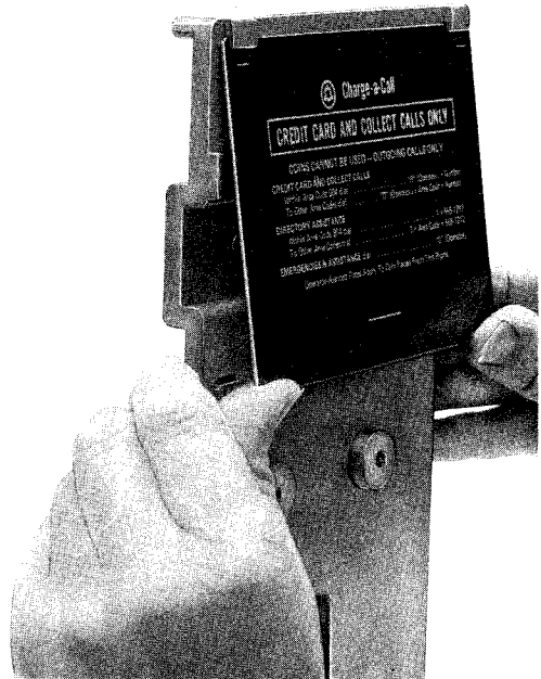
Fig. 12—Installing Instruction Card On Rear Panel Support of KS-22284 Backboard
