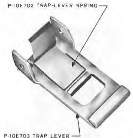
Fig. 9 - Trap-Lever Spring Assembled on Trap Lever
