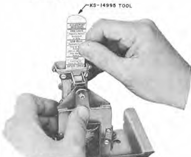
Fig. 4—Trap and Vane Release Test
