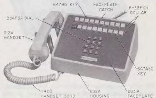
Fig. 2—2831CT (MD) Telephone Set, Assembled
