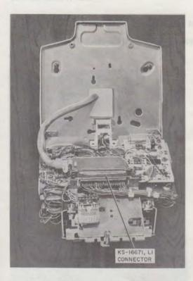
Fig. 3—853AM or 2853AM Telephone Set With Hinged Chassis Assembly in Lowered Position
