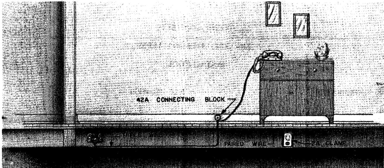
**Fig. 2 — Typical Installation of 702B Telephone Set**
