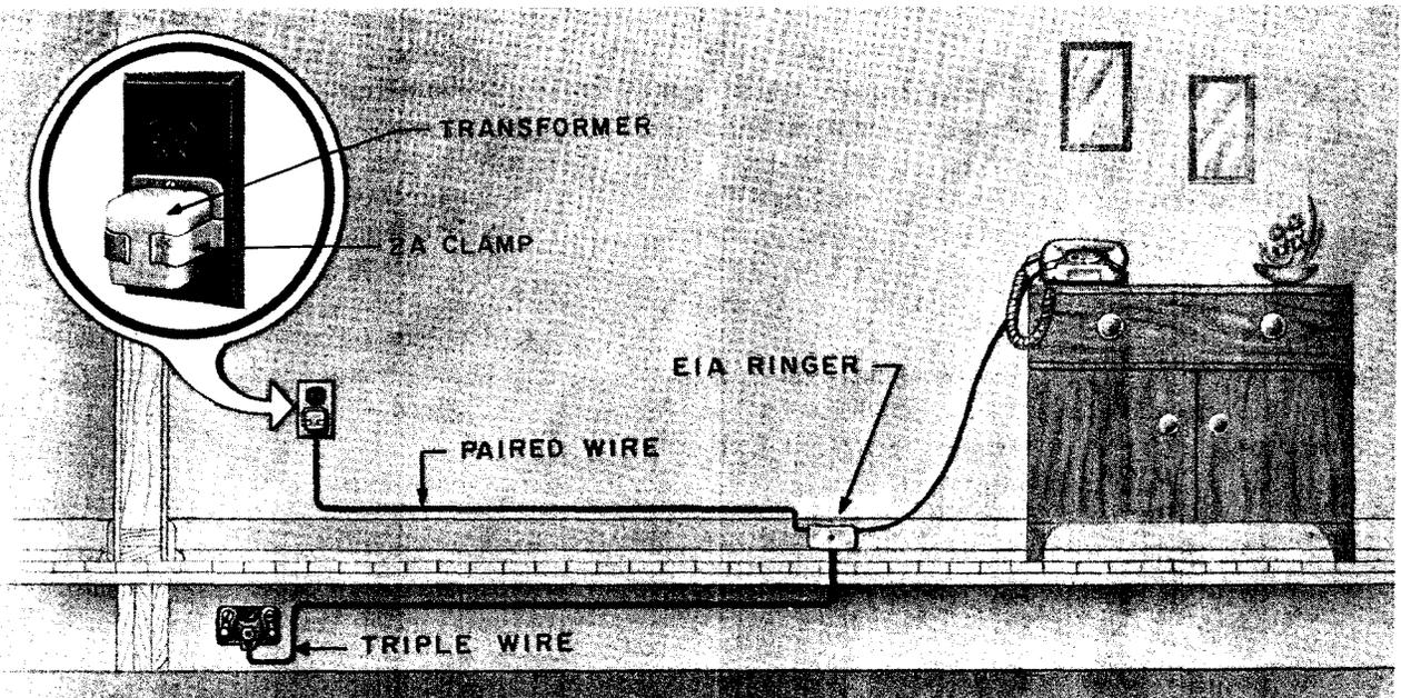
Fig. 1 — Typical Installation of 701B Telephone Set
