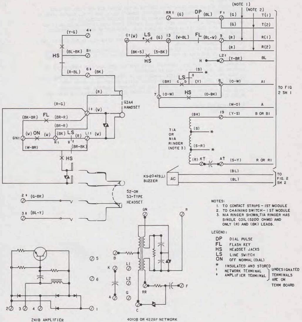
Fig. 1—636CA and 637DA Telephone Set, Connections
