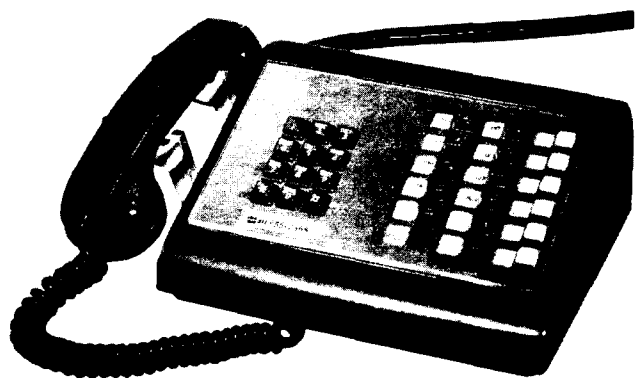
Fig. 2—Typical Nonmodular Telephone Set Using 590 or 650 Series Keys
