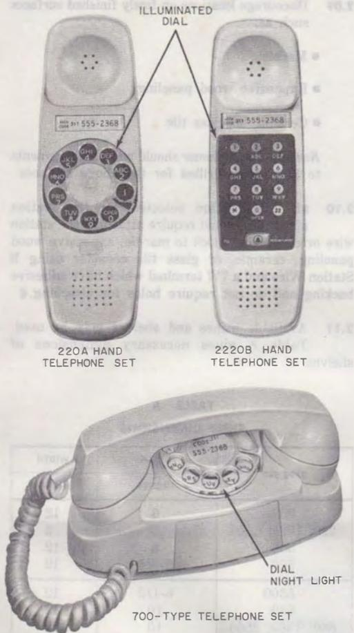
**Fig. 2—Hand Telephone Sets and Telephone Set With Illuminated Dial Feature**
