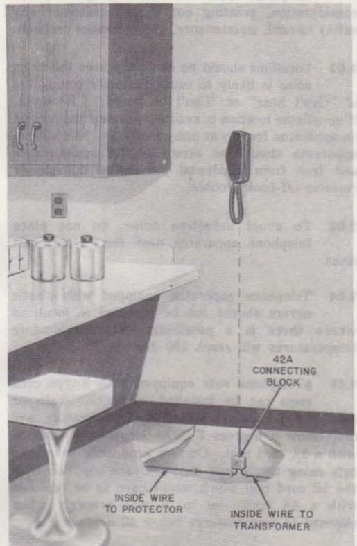
**Fig. 3—Typical Installation of AC1 Telephone Base With 220A Hand Telephone Set**
