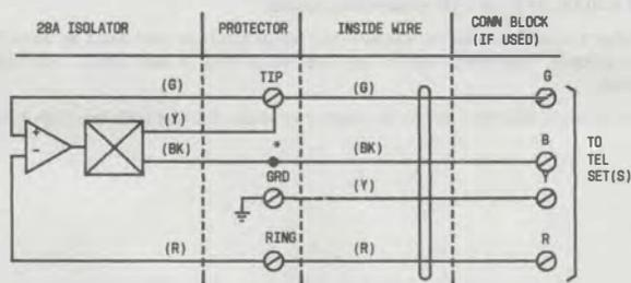
\* SPLICE TOGETHER USING 700-TYPE CONNECTOR OR EQUIVALENT
