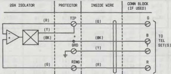
\* SPLICE TOGETHER USING 700-TYPE CONNECTOR OR EQUIVALENT
