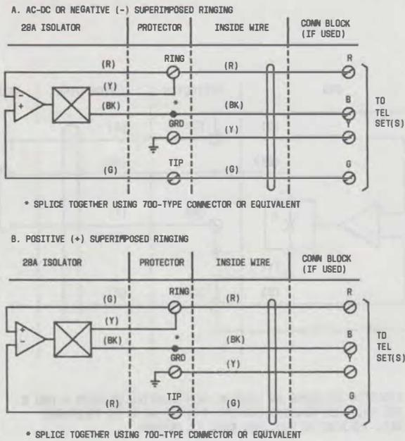
Fig. 3—28A Isolator Connections for Ring Parties (4-Conductor Wiring)
