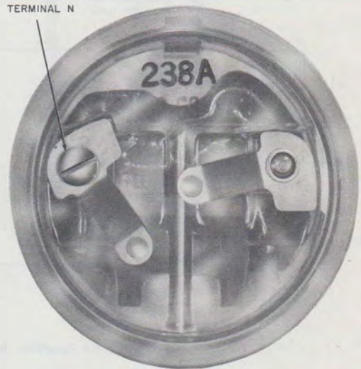
Fig. 2—238A Amplifier, Showing Typical Terminal N Location
