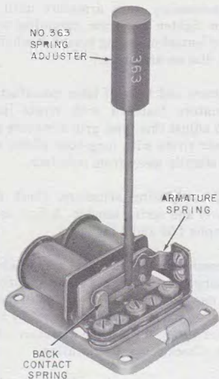
Fig. 18—Adjusting Armature Spring, 7-Type Buzzer
