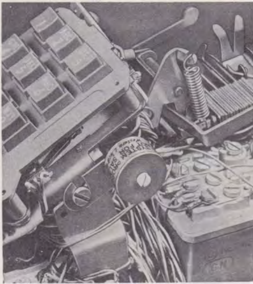
Fig. 13—KS-20419L1 Buzzer Mounted on TOUCH-TONE® Dial Mounting Screw
