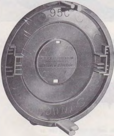
Fig. 4—95C (Current Model)—Similar in frontal appearance to the 95C (early model). Equipped with ribs which provide frictional fit to dial mounting bracket on sets having 2 and 3 point suspension.
