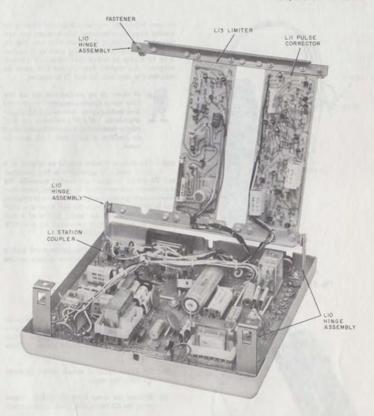
Fig. 3—KS-20721 Station Coupler Showing Optional Circuit Packs Mounted
