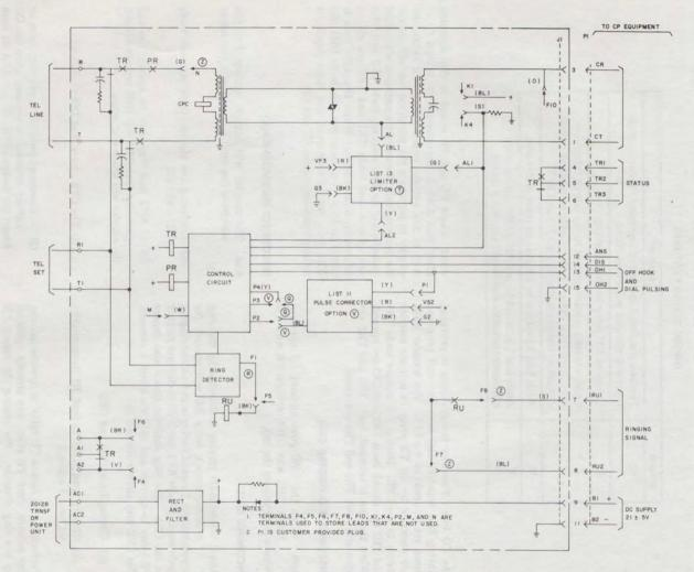
Fig. 7\$KS-20721 Station Coupler, Internal Wiring Options
