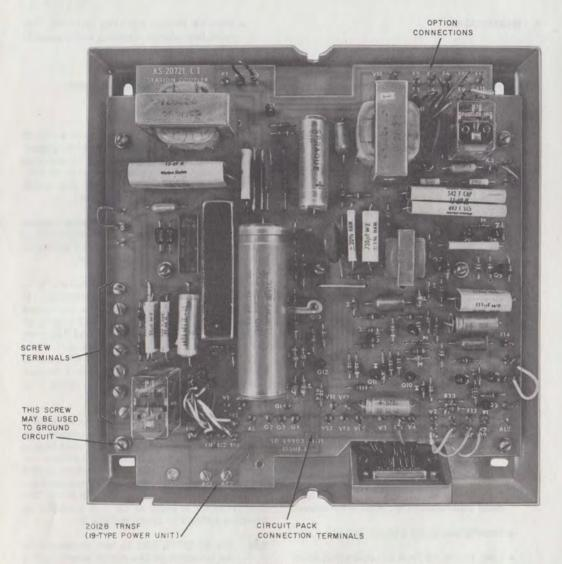
Fig. 2-KS-20721, List 1 Station Coupler, Cover Removed
