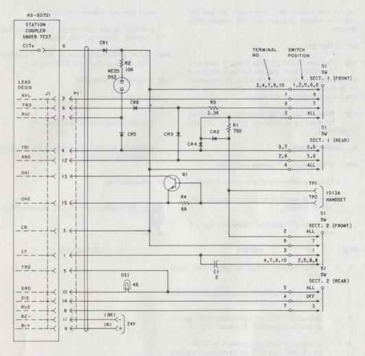
Fig. 8-KS-20721, List 15 Test Set Schematic
