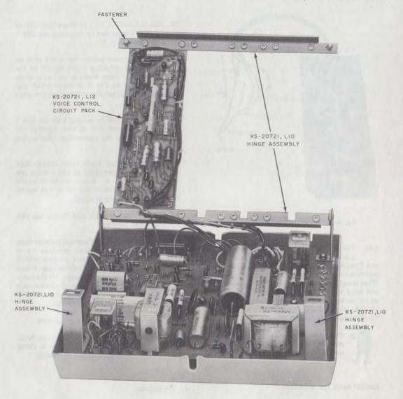
Fig. 3-#KS-20721, List 2 Station Coupler With Optional Circuit Pack #
