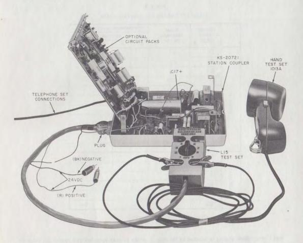
Fig. 5—KS-20721 Station Coupler with KS-20721, List 15 Test Set and 1013A Hand Test Set
