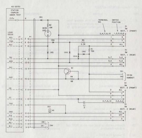
Fig. 7-KS-20721, List 15 Test Set Schematic
