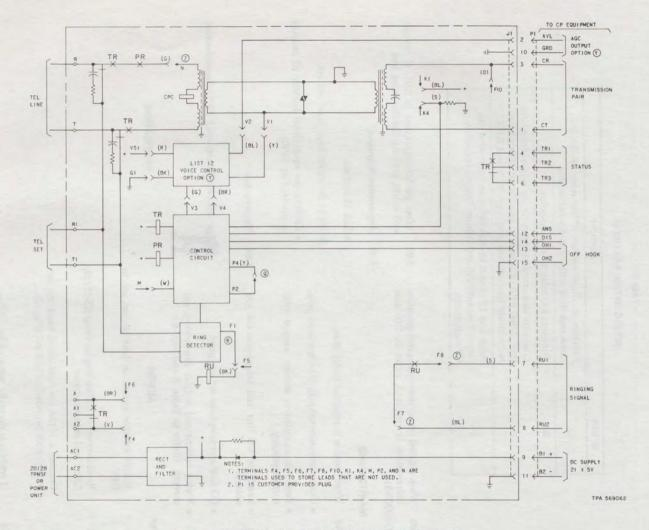
Fig. 6—♦KS-20721 Station Coupler, Internal Wiring Options (
