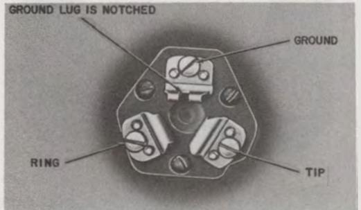
Fig. 22—Connections for KS-8420 and KS-8421 Jacks (MD)
