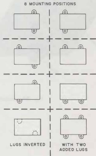
Fig. 28—KS-19316, List 6, Housing Box Showing Reversible Mounting Lugs
