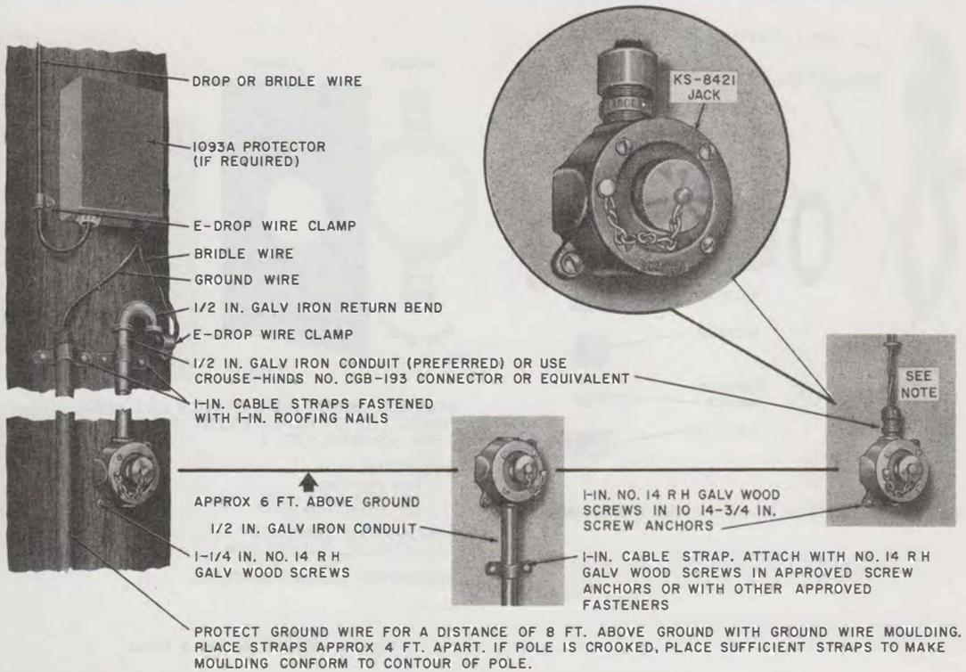
NOTE: WHEN TWISTED PAIR OR TRIPLE WIRE IS USED, PLACE A LAYER OF RUBBER TAPE BETWEEN THE CONDUCTORS WHERE THEY ENTER THE RUBBER PLUG OF THE CONNECTOR SO THAT WHEN THE CONNECTOR CAP IS TIGHTENED THE HOLE WILL BE EFFECTIVELY SEALED.
