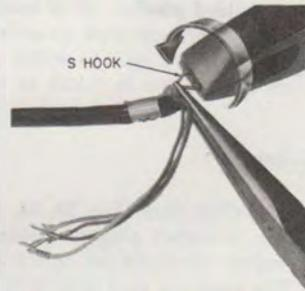
Fig. 36—Bending S Hook
