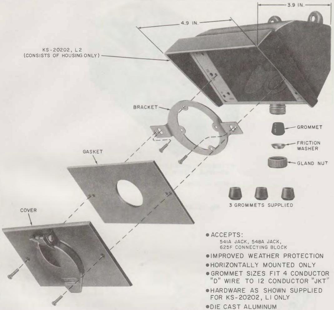
Fig. 23—♦Assembly of KS-20202, List 1 and 2 Waterproof Housing♦
