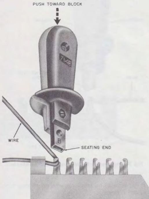
**Fig. 3—Preparation for Looping Termination**
