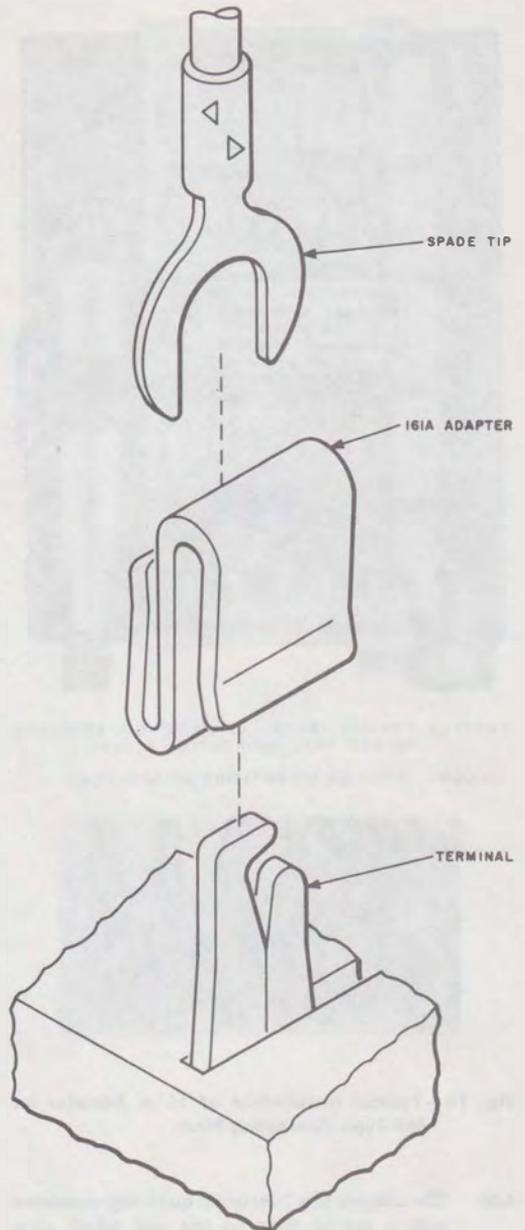
**Fig. 9—161A Adapter, Installation Detail**
