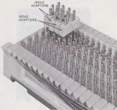
Fig. 12—Typical Installation of 183A2 Adapters on 66B-Type Connecting Block
