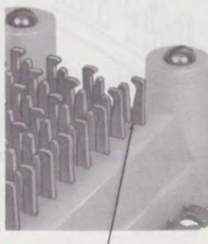
**Fig. 17—Gap Spread Distorted**
