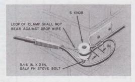
Fig. 8—First Attachment, Corner Bracket Using S Knob
