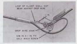
Fig. 7—First Attachment, Corner Brocket
