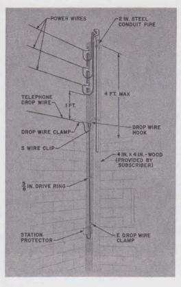
Fig. 13—Drop Wire Attached to Subscriber Pole
