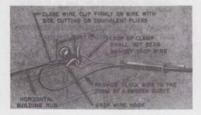
Fig. 3—First Attachment, Drop Wire Hook
