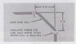
Fig. 17—Spacing Insulated Screw Eye When Changing
