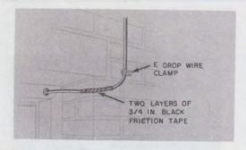
Fig. 19—Last Attachment, Building Entrance Slopes
