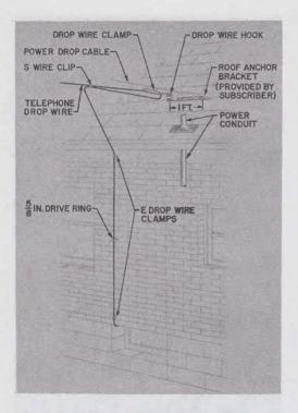
Fig. 12—Drop Wire Attached to Roof Anchor Bracke
