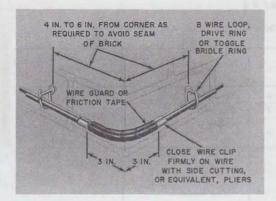
Fig. 14—Spacing Attachments at Outside Corner of Building
