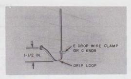
Fig. 20—Last Attachment, Building Entrance Hole Does Not Slope Upward From Outside
