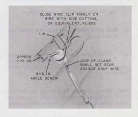
Fig. 1—First Attachment, Horizontal Run
