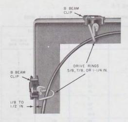
Fig. 18—B Beam Clips
