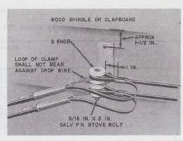
Fig. 6—First Attachment, House Bracket Horizontal
