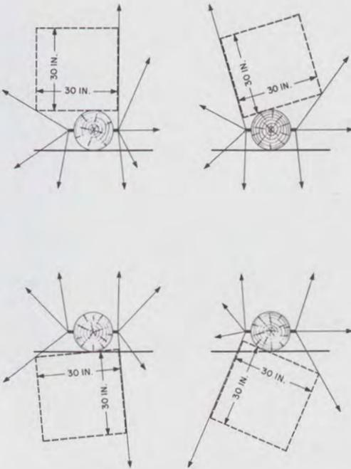
Fig. 4—Climbing Space When Drops are Attached Directly to Pole
