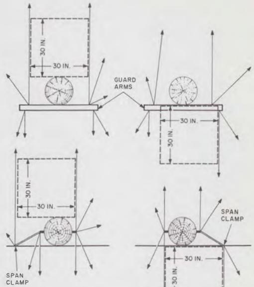
Fig. 5—Use of Guard Arm or Span Clamp to Maintain Climbing Space
