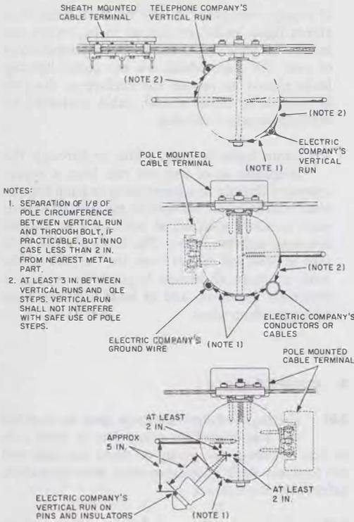
Fig. 1—Typical Vertical Run Clearances
