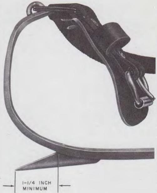
Fig. 21—Gaff Sharpened to Minimum Length
