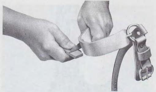
Fig. 18—Removing Burrs From Bottom Cutting Edge
