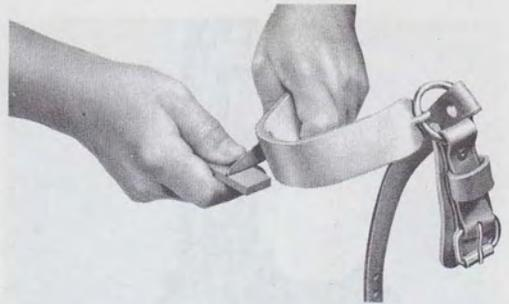
Fig. 18—Removing Burrs From Bottom Cutting Edge
