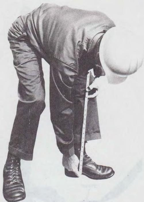
Fig. 8—Measuring for Climber Length
