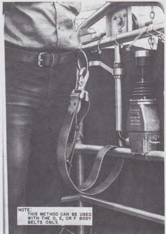
Fig. 9—Method of Using D, E, or F Body Belt With Safety Strap in TELSTA Aerial Lift
