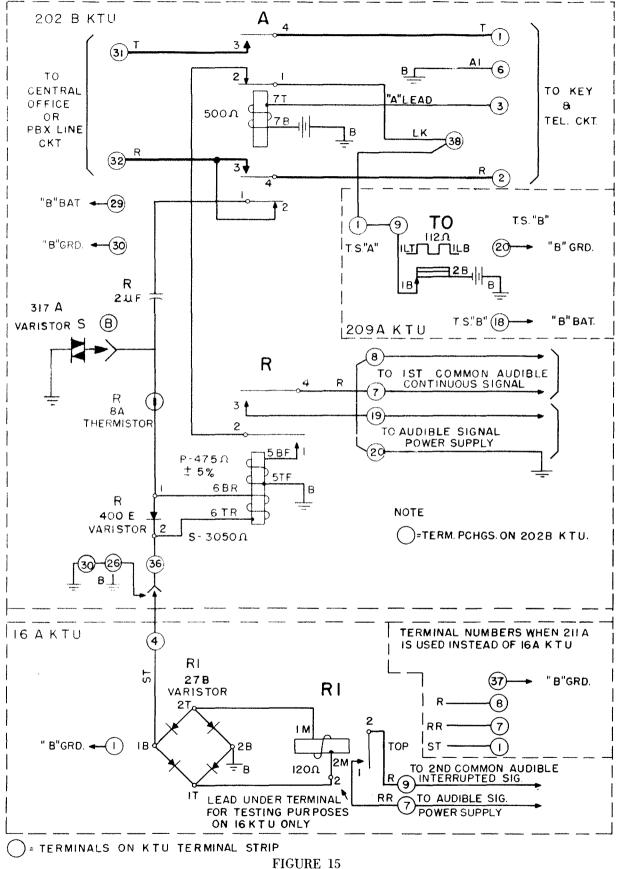
Central Office or PBX Line Circuit — Common Audible Signal — 16A, 202B, 209A, and 211A Key Telephone Units
