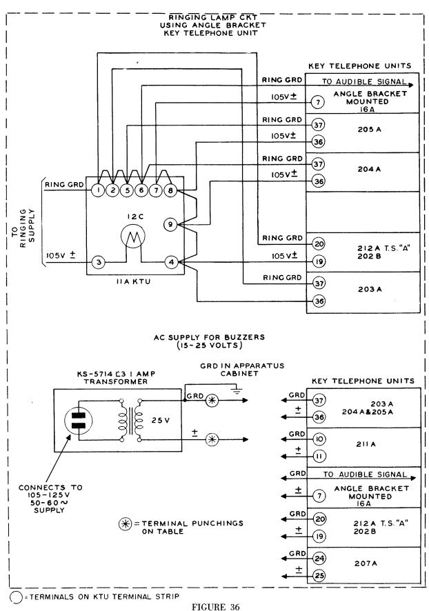
Ringing Lamp Circuit and AC Supply for Buzzers (15 to 25 Volts) — 11A Key Telephone Unit and KS-5714, L3 Transformer
