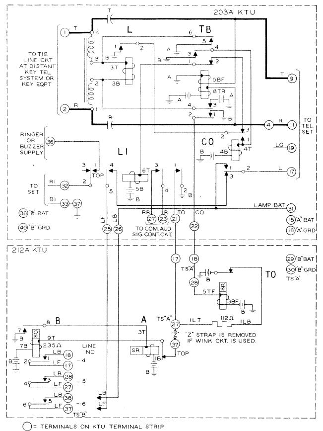
FIGURE 11 Automatic Tie Line Circuit – 203A and 212A Key Telephone Units
