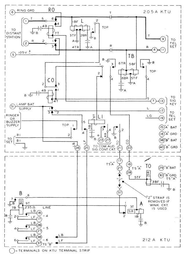
FIGURE 37 Station Line Circuit --- 205A and 212A Key Telephone Units
