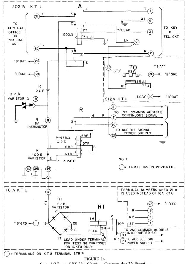
Central Office or PBX Line Circuit — Common Audible Signal — 16A, 202B, 211A, and 212A Key Telephone Units
