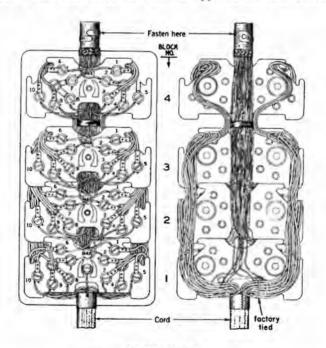
FIGURE 10 Four No. 44A Connecting Blocks. One Nos. 101A and 101C Covers Required
