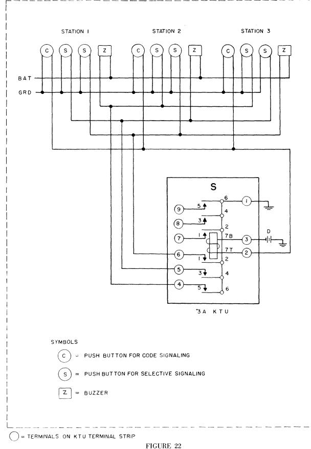
FIGURE 22 Code and Selective Signaling — 3A Key Telephone Unit
