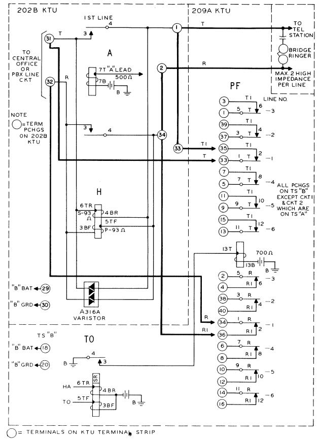
FIGURE 32 Power Failure Circuit – 202B, and 209A Key Telephone Units
