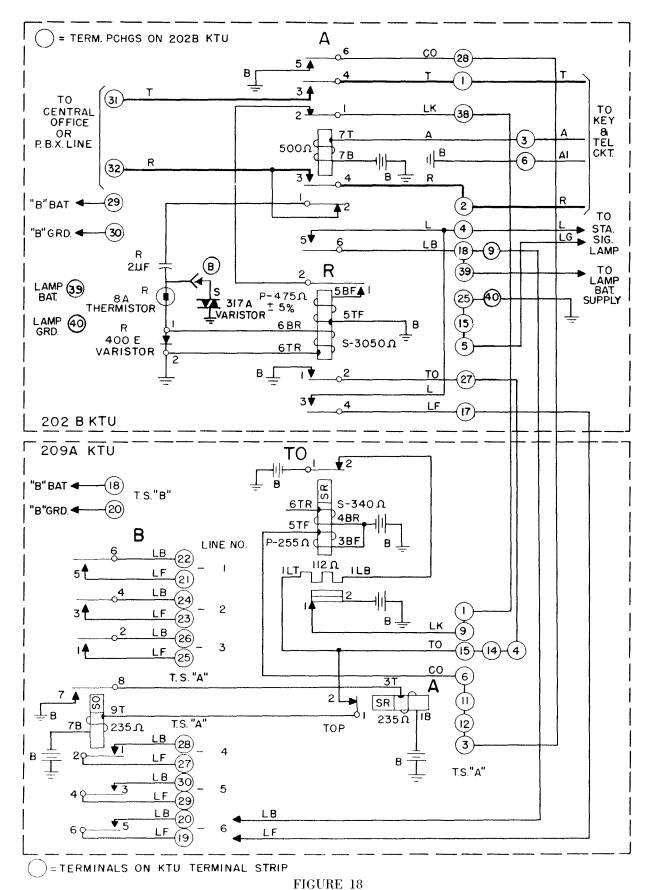
Central Office or PBX Line Circuit — Lamp Flashing, Incoming Visual Signal, Time-out, and Busy Signal Circuit — 202B and 209A Key Telephone Units
