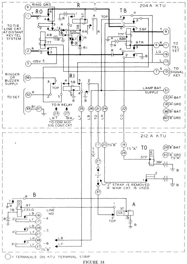
Ringdown Tie Line Circuit - 204A and 212A Key Telephone Units
