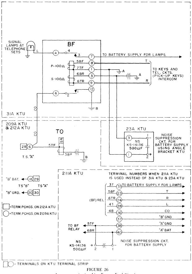
Intercommunicating Line Battery Feed Circuit — 23A, 31A, 209A, 211A, and 212A Key Telephone Units
