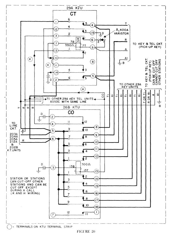
Cut-Through and Control Circuit for Automatic Cut-off (H and K Wiring) – 26B and 29A Key Telephone Units
