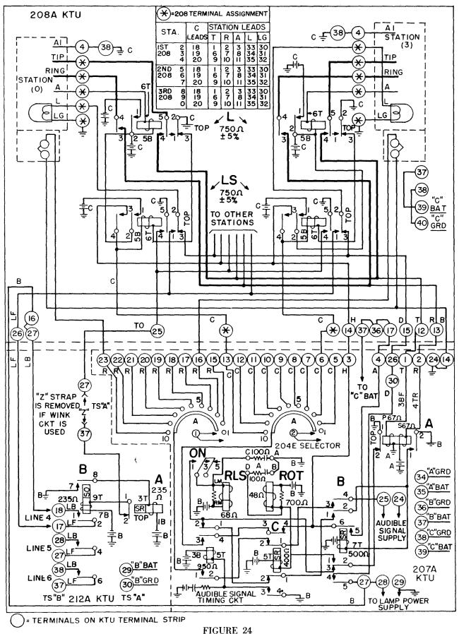
Dial Selective Intercommunicating Line Circuit with Flashing Line Lamps — 207A, 208A, and 212A Key Telephone Units
