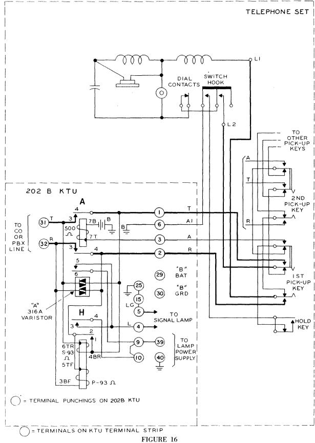
Central Office or PBX Line Hold Circuit — 202B Key Telephone Units
