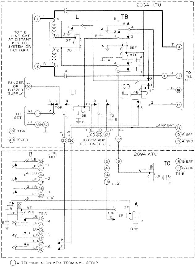
FIGURE 12 Automatic Tie Line Circuit --- 203A and 209A Key Telephone Units
