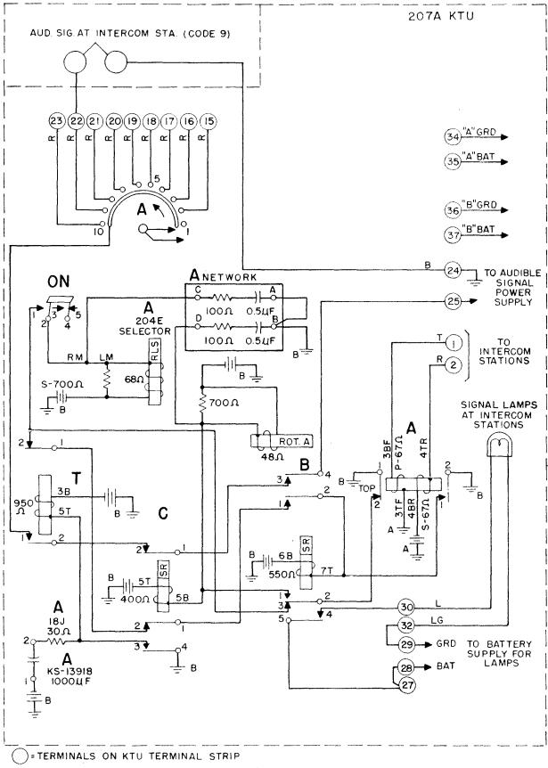
FIGURE 23 Dial Selective Intercommunicating Line Circuit --- 207A Key Telephone Unit
