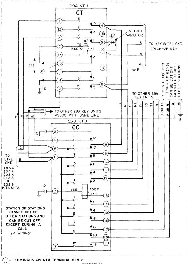
FIGURE 19 Cut-Through and Control Circuit for Automatic Cut-off (K Wiring) – 26B and 29A Key Telephone Units
