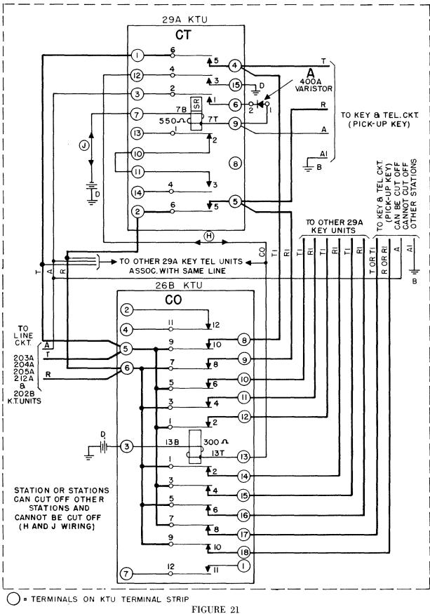
Cut-Through and Control Circuit for Automatic Cut-off (H and J Wiring) — 26B and 29A Key Telephone Units
