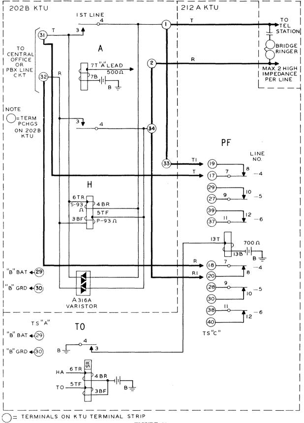
FIGURE 31 Power Failure Circuit – 202B, and 212A Key Telephone Units
