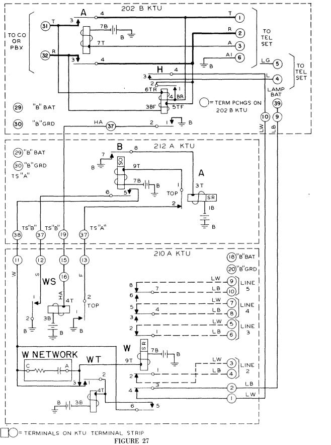
Lamp Winking Circuit — 202B, 210A, and 212A Key Telephone Units
