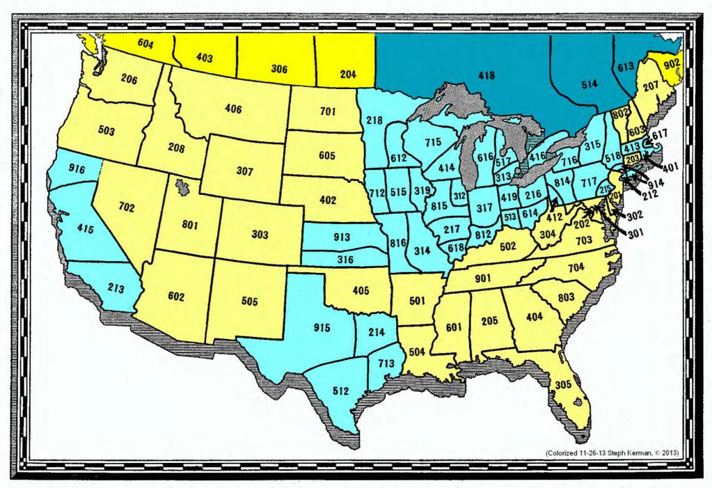
Figure I. Map of U.S.A. (and adjacent Canadian territories) showing toll numbering plan areas and tentative three-digit area codes. (Courtesy Bell System) (from Automatic Electric Technical Journal, Oct. 1948)
