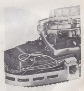
Fig. 16—2702B2M Telephone Set Base With Mounting
