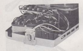
Fig. 14—2554B2M Telephone Set Base With Handset Jack Installed
