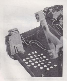
Fig. 18—500D2M or 2500D2M Telephone Set Base
