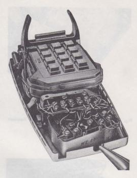
Fig. 19—Modifying 2554B-Type Telephone Set Base to Accommodate Handset Jack
