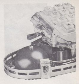
Fig. 15—2702B2M Telephone Set Base With Handset Jack Installed
