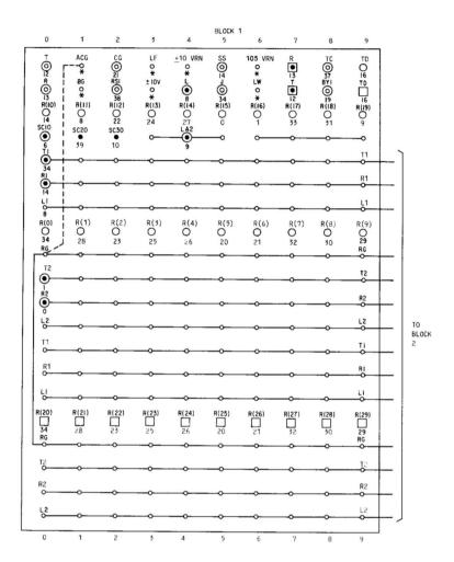
Fig. 17—♦Connecting Block Terminal Identification (Sheet 1 of 3)€
