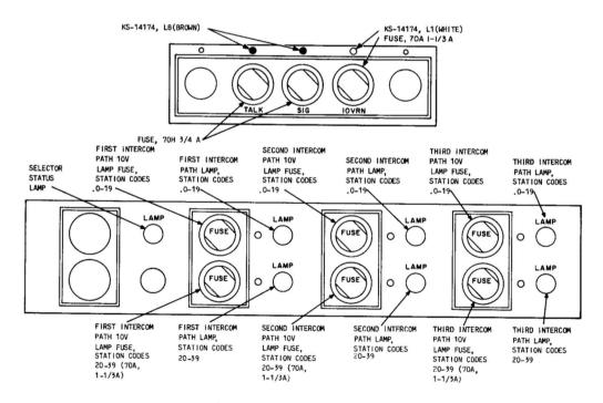
Fig. 3—Fuse and Lamp Arrangement, 626A Panel
