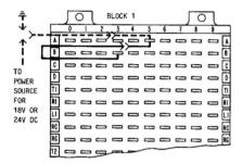
OPTION FOR 10V AC BUZZER UNINTERRUPTED SIGNAL OR FOR 18V DC, 24C DC, GROUND OR AS REQUIRED FOR SIGNALING PURPOSES OTHER THAN PROVIDED (EXTERNAL POWER SOURCE MAY BE REQUIRED).
