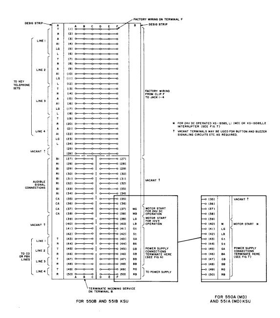
Fig. 4— Terminal Layout of Connecting Block on 550/551A and B KSUs (MD) Showing Installer Connections for Incoming Lines and Stations
