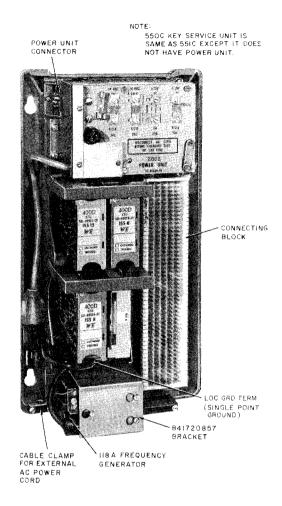
Fig. 1---▶551C KSU With Frequency Generator
