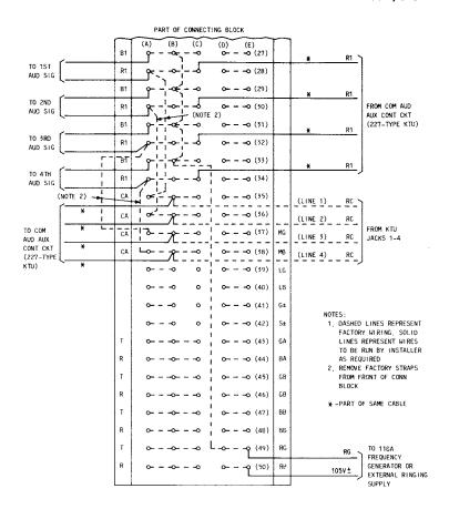
Fig. 9—Connections for Common Audible Auxiliary Control on 550/551C KSUs
