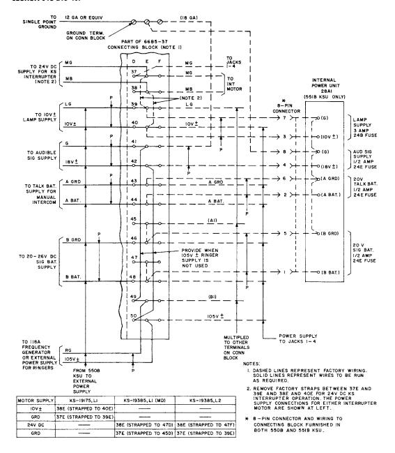
Fig. 6—Power Supply Connections for 550/551B KSUs (MD)
