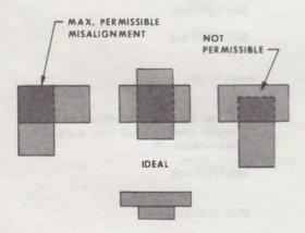
Fig. 11—Contact Alignment
