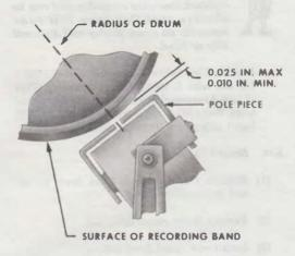
Fig. 12—Erase Coil Clearance
