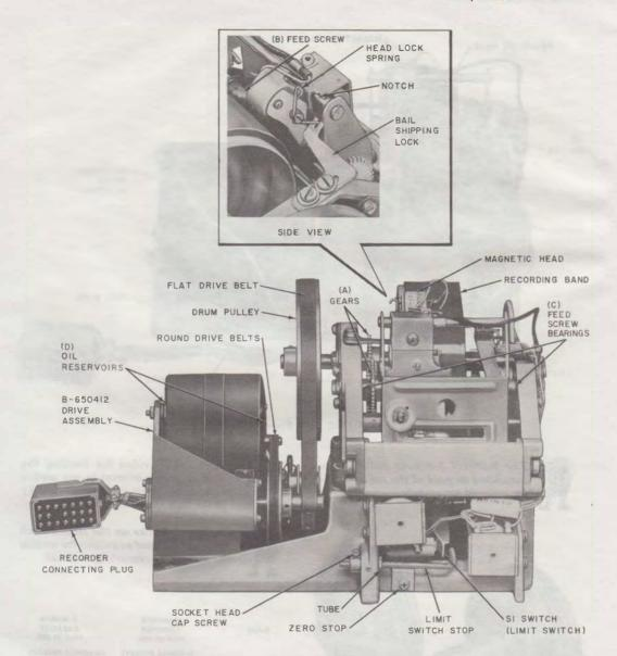
Fig. 6-KS-16765, List 3 Recorder, Front View
