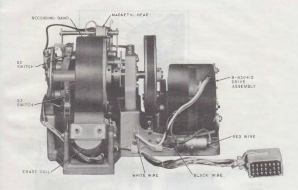
Fig. 7—KS-16765, List 3 Recorder, Rear View
