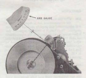
Fig. 14—Magnetic Head Pressure
