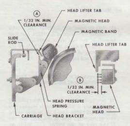
Fig. 13—Head Lifter Tab Clearance
