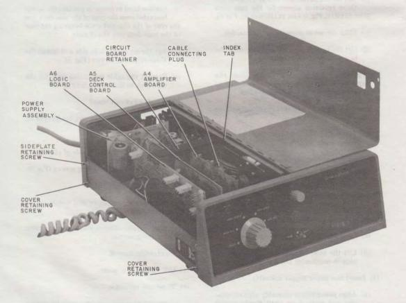
Fig. 4—Top Cover Removed, Internal View of Components
