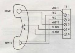
Fig. 8—Handset Connections
