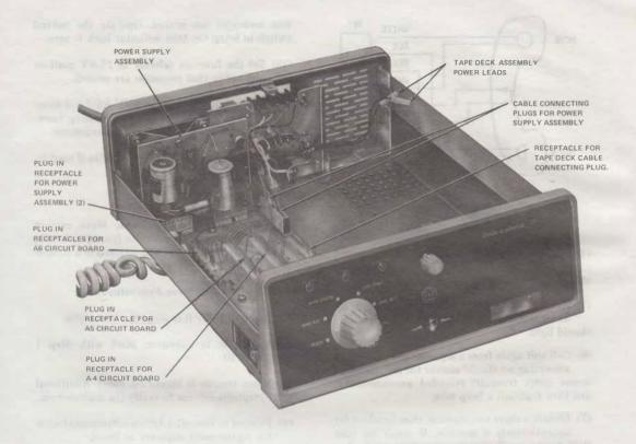
Fig. 7—Top Cover, Circuit Boards and Tape Deck Removed
