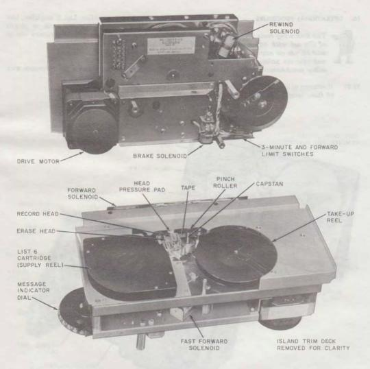
Fig. 9—KS-19245, List 3 Recorder Front and Rear Views
