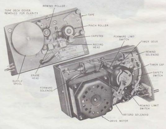
Fig. 8—KS-19245, List 2 Recorder Front and Rear Views
