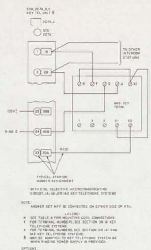
Fig. 6—KS-19245, List 1 Telephone Set Connections (Sheet 3 of 3)
