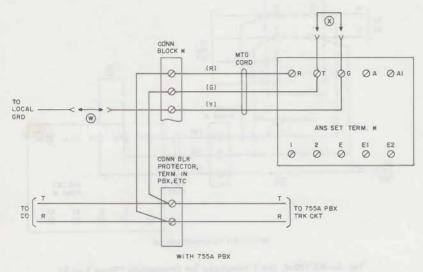
Fig. 6—KS-19245, List 1 Telephone Set Connections (Sheet 2 of 3)
