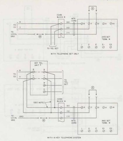
Fig. 6—KS-19245, List 1 Telephone Set Connections (Sheet 1 of 3)
