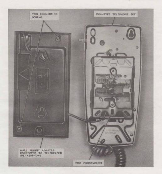
Fig. 13— Rear View of TELEHELPER Speakerphone With Wall Mount Adapter Attached and 2554-Type Telephone Connected on 730B Phonemount
