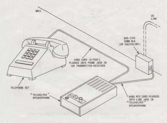
Fig. 6—Recommended Installation for Single Line Modular Desk Type Telephone Set
