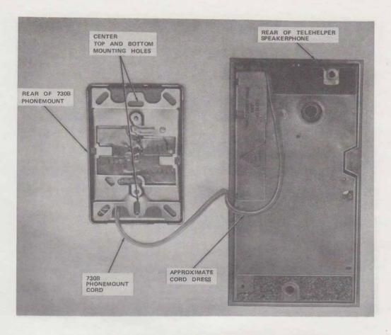
Fig. 11 — Approximate Cord Dress of 730B Phonemount Cord With Telephone Location Right of TELEHELPER Speakerphone
