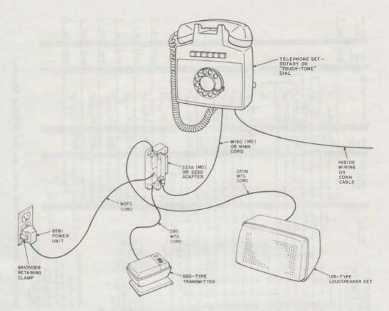
Fig. 1—4A Speakerphone System Arrangement, 6-Button Wall Telephone Set
