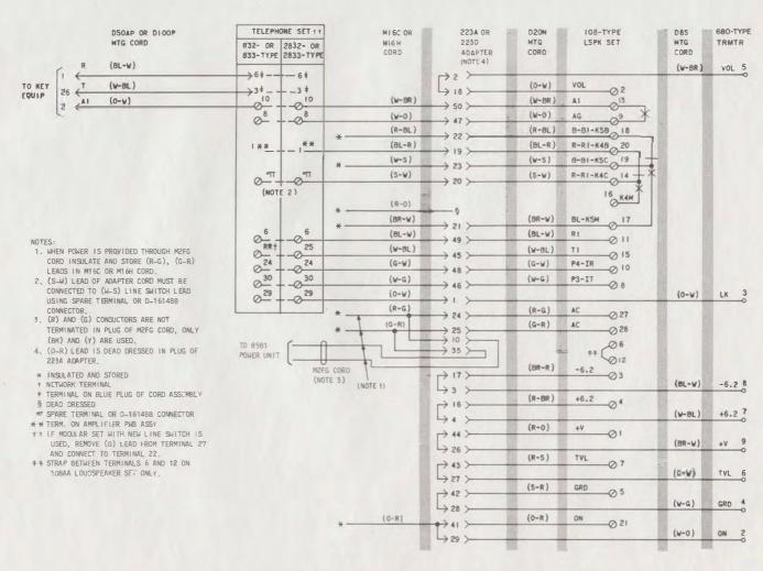
Fig. 2---♦4A Speakerphone System Arrangement, Connections to 10- or 20-Button Telephone Set♠
