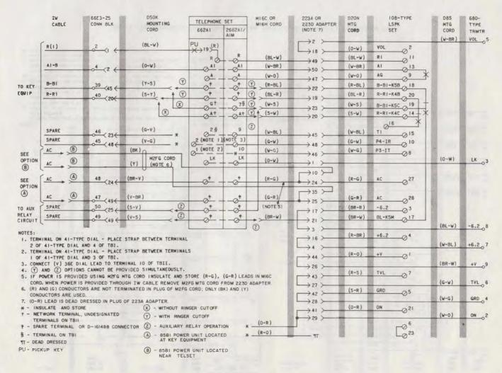
Fig. 4—Speakerphone Connections, Adapter Terminated In Set
