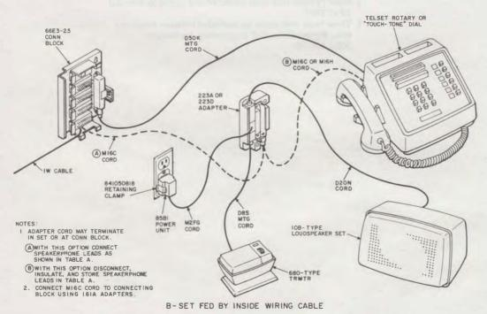
Fig. 1—Speakerphone Arrangement, 662- or 2662- Type Telephone Set
