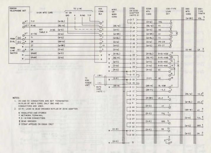
Fig. 4—₱Typical Grandfathered 4A Speakerphone System Arrangement, Connections to 2660A1 (MD) Telephone Set◀
