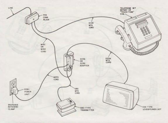
Fig. 1—₱Typical Grandfathered 4A Speakerphone System Arrangement, 660A1 (MD) or 2660A1 (MD) Telephone Sets Using 223A (MD) or 223D Adapter♥
