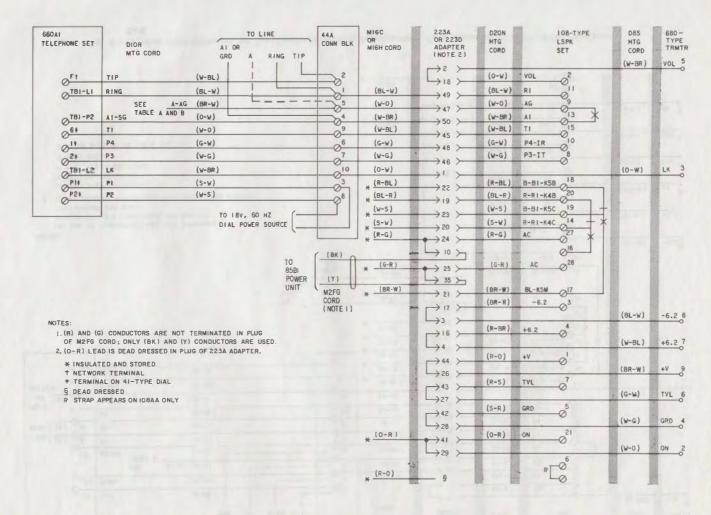
Fig. 3—₱Typical Grandfathered 4A Speakerphone System Arrangement, Connections to 660A1 (MD) Telephone Set♥
