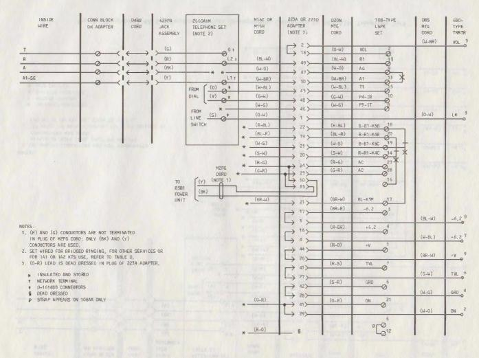
Fig. 5-PTypical Grandfathered 4A Speakerphone Arrangement, Connections to 2660A1M Telephone Set
