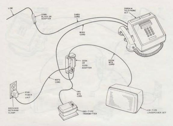
Fig. 2—Registered or Typical Grandfathered 4A Speakerphone System Arrangement, 2660A1M Telephone Set Using 223A (MD) or 223D Adapter€
