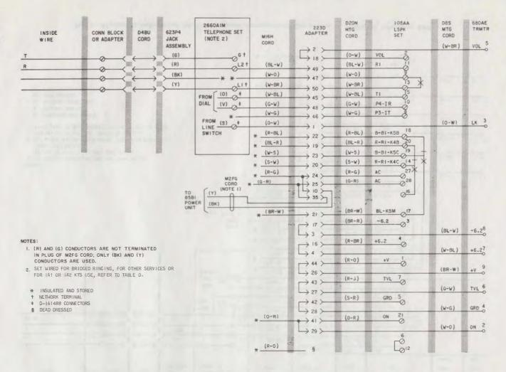
Fig. 6—PRegistered 4A Speakerphone System Arrangement, Connection to 2660A1M Telephone Set®
