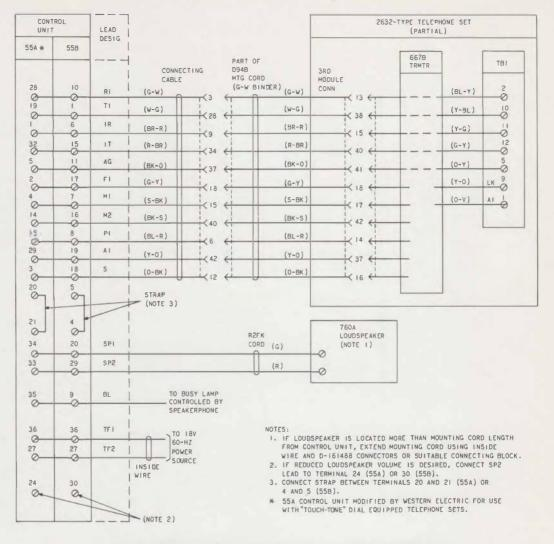
Fig. 1—2632-Type Telephone Set, Connection For 3-Type Speakerphone
