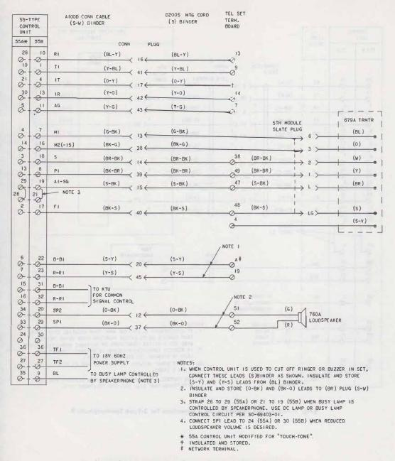
Fig. 2—2631DA Telephone Set Connections for 3-Type Speakerphone
