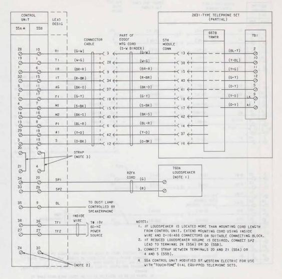
▶Fig. 1—2631-Type Telephone Set, Connections for 3-Type Speakerphone ◆
