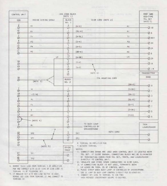
Fig. 1—832- and 833-Type Telephone Sets—3-Type Speakerphone Connections
