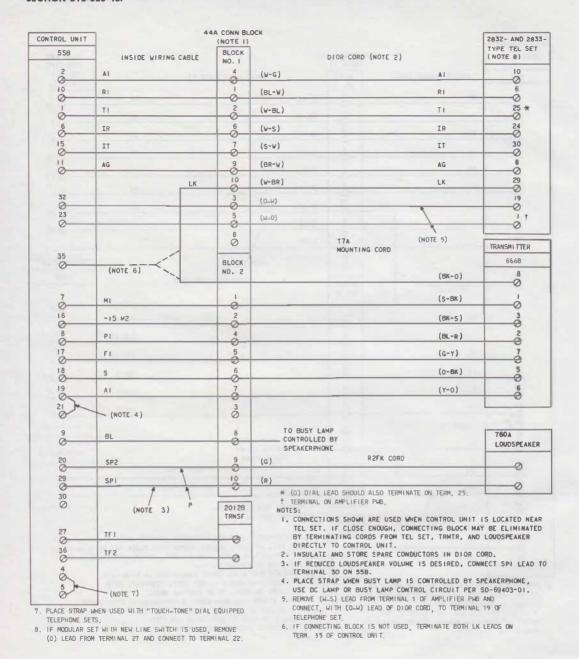
Fig. 2—2832- and 2833-Type Telephone Sets—3-Type Speakerphone Connections
