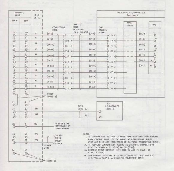
Fig. 3—2632-Type Telephone Set, Connections to 3-Type Speakerphone System
