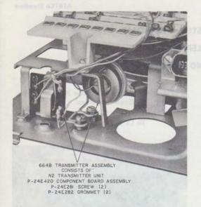
Fig. 2-664B Transmitter Assembly Installed
