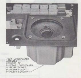
Fig. 1—762A Loudspeaker Assembly Installed
