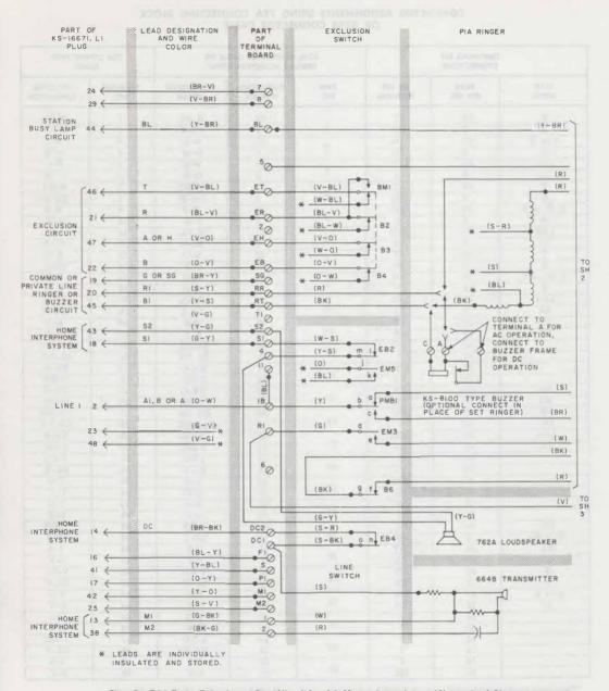
Fig. 3—754-Type Telephone Set Wired for 1A Home Interphone (Sheet 1 of 3)
