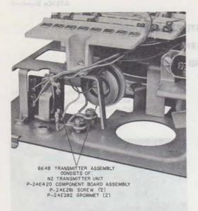
Fig. 2-664B Transmitter Assembly Installed
