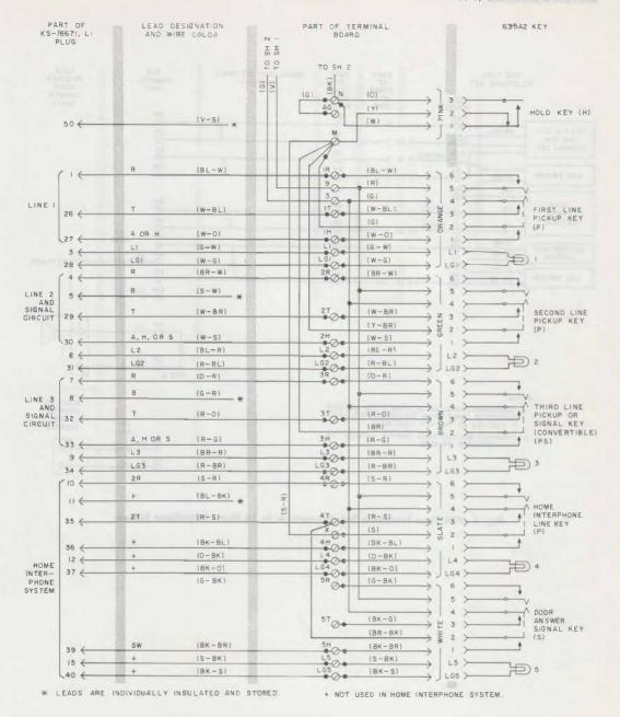
Fig. 3-754-Type Telephone Set Wired for 1A Home Interphone (Sheet 3 of 3)
