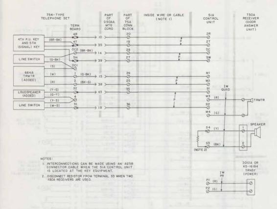
Fig. 4—754-Type Telephone Set, Connections to 1A Home Interphone System
